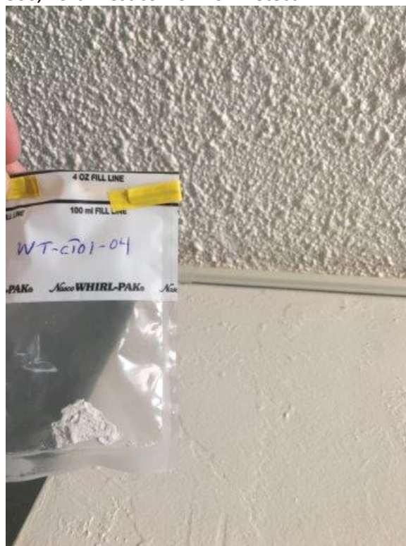
WT-CT01-04- Popcorn Ceiling Texture- Room 307, corner of kitchen and hallway-8% Chrysotile
