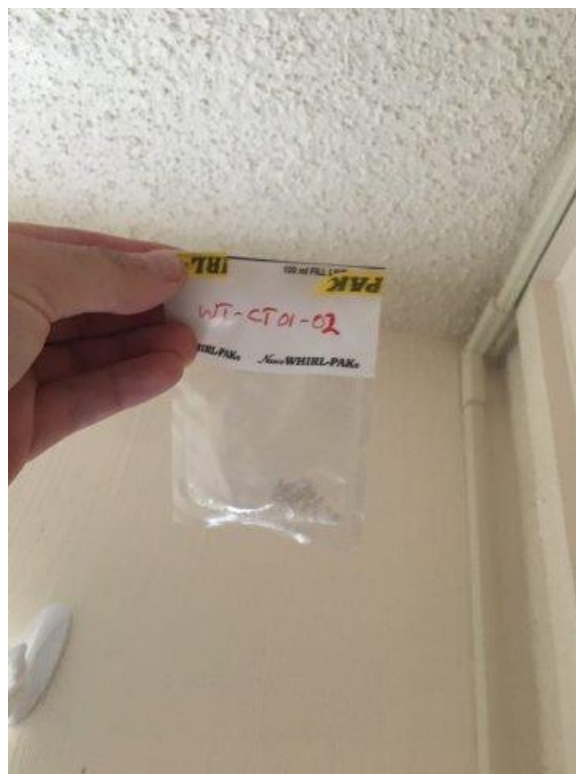
WT-CT01-02-Popcorn Ceiling Texture- Room 306, northwest corner-Non-Detect
